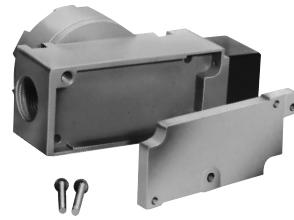
Catalog Listing **LSXZ4022** adapter plate enables the explosion-proof LSX to be mounted on existing HDLS mounting holes. The LSX has a recessed back into which the adapter plate fits and mounts, using two screws (furnished).
